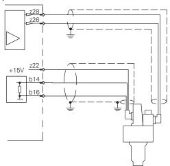
Note: If valves are fitted with the "B" type LVDT, the screen will be grounded at the valve end by the shell of the connector.
