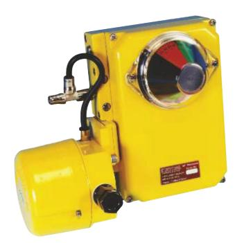
The optional Kinetrol I/P Controller is mounted in place of the standard diaphragm housing on the side of the positioner case. The positioner can still be mounted in any orientation and gives an angular output position which is proportional to the input current control signal between 4-20mA.
