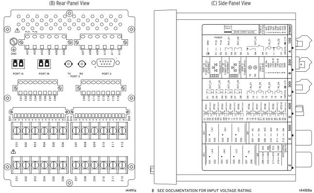
Figure 23 Dual-Fiber Ethernet, Fast Hybrid 4 DI/4 DO, 10 RTDs, 3 ACI/2 AVI, 4 ACI/3 AVI
