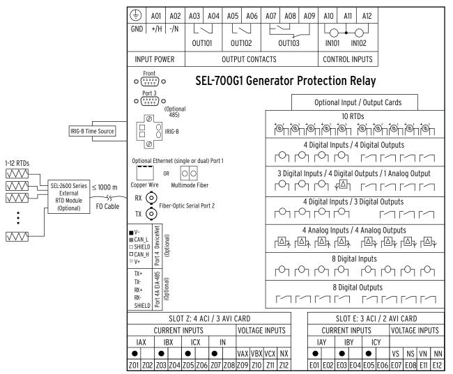
Figure 15 Typical Connection Diagram
