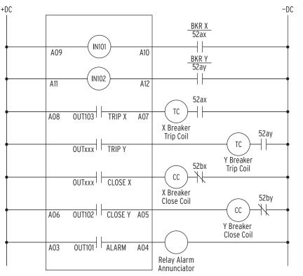
Figure 22 SEL-700GW Typical DC External Connections
