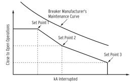
Figure 8 Breaker Contact Wear Curve and Settings
