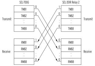
Figure 13 MIRRORED BITS Transmit and Receive Bits
