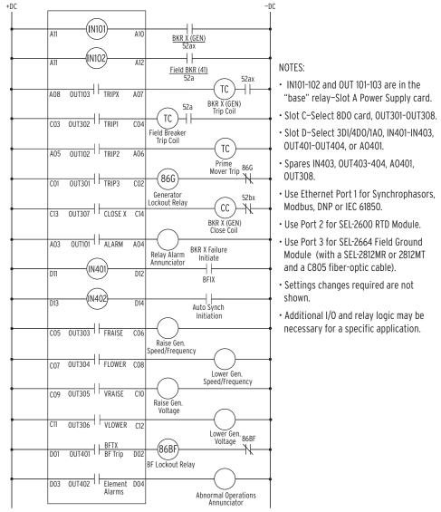
Figure 17 SEL-700G1 Typical DC External Connections
