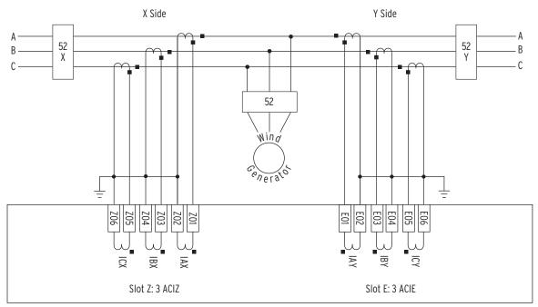
Figure 21 SEL-700GW Dual Feeder AC Current Connections
