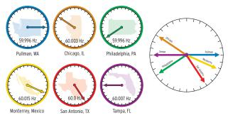
Figure 6 View of System Angle at Multiple Locations
