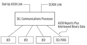
Figure 9 Example Communications System
