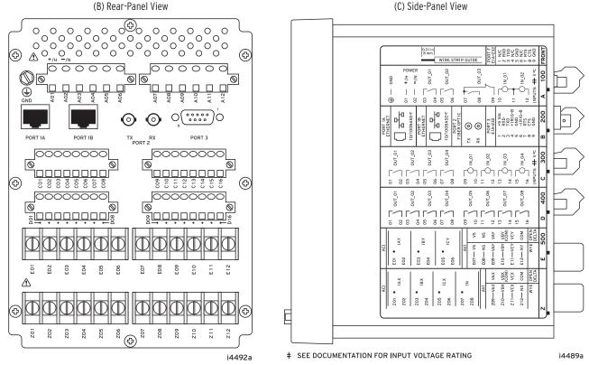
Figure 24 Dual Copper Ethernet, 4 DI/4 DO, 8 DO, 3 ACI/4 AVI, 4 ACI/3 AVI
