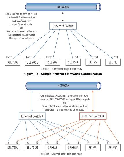
Figure 11 Simple Ethernet Network Configuration With Dual Redundant Connections (Failover Mode)
