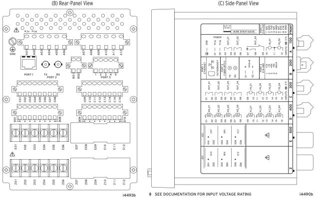
Figure 25 Copper Ethernet, 4 DI/4 DO, 4 AI/4 AO, 3 ACIE, 3 ACIZ
