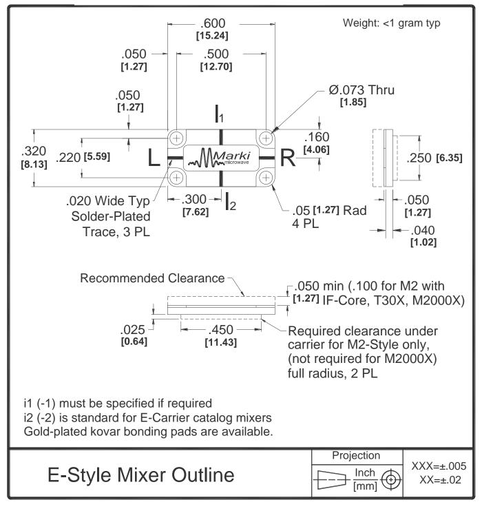
E-Carrier I/O trace finish is reflowed Sn63/Pb37 solder plate over Cu. E-Carrier is Half Hard Brass, plated Electroless Nickel 150-250 μ-inches, followed by Nickel Flash. Click on links for suggested System layout and Carrier Mounting notes.
