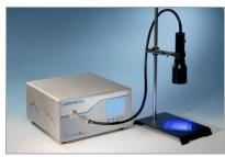
**Rod Lenses** Shown: BlueWave 200 with 8 mm rod lens stand and clamp PN 38968 (rod lenses require an 8 mm lightguide) 2" x 2" Area (~100 mW/cm²) PN 38699 5" x 5" Area (~30 mW/cm<sup>2</sup>) PN 38698
