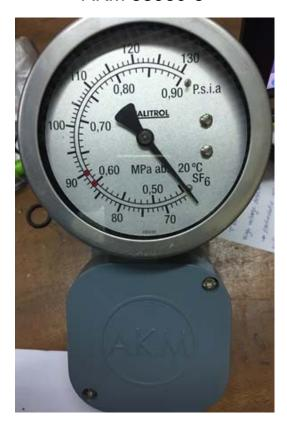
Part No. & Model of SF6 Gas Density Monitor
