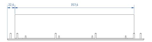
Front Panel: **Panelmount "PMA"** (5 mm aluminium, powder-coated RAL 7035)
