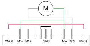
FIGURE 10. MDC2230S/MDC2460S wiring diagram
