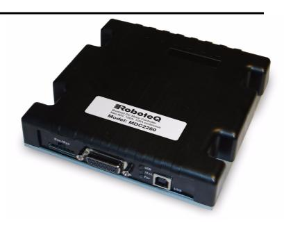
Roboteq's MDC2xxx controller is designed to convert commands received from an RC radio, Analog Joystick, wireless modem, PC (via RS232 or USB) or microcomputer into high voltage and high current output for driving one or two DC motors. Designed for maximal ease-of-use, it is delivered with all necessary cables and hardware, and is ready to use in minutes. Using CAN bus, up to 127 controllers can be networked at up to 1Mbit/s on a single twisted pair.
