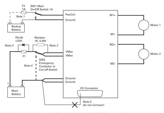
FIGURE 8. Powering the controller. Thick lines identify **MANDATORY** connections
