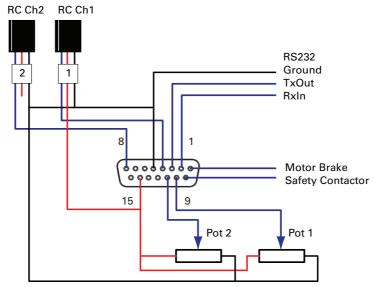
FIGURE 13. Factory default pins assignment
