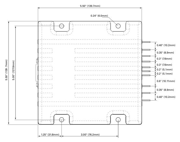
FIGURE 17. MDC2xxx top view and dimensions
