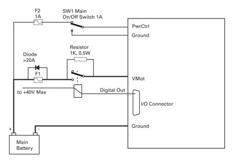
FIGURE 9. Contactor wiring diagram
