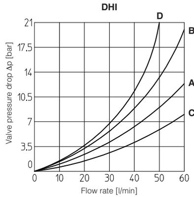
**7 OPERATING LIMITS** based on mineral oil ISO VG 46 at 50°C
