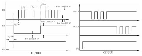
Figure 11: Sequence chart of control signals
