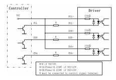
Figure 3: Connections to open-collector signal (common-anode)
