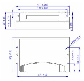
Figure 1: Mechanical specifications
