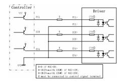
Figure 4: Connection to PNP signal (common-cathode)
