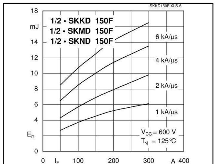
Fig. 6 Typ. turn-off energy dissipation per pulse
