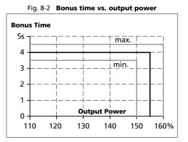
Bonus Power<sup>®</sup> is available as soon as power comes on and immediately after the end of an output short circuit.
