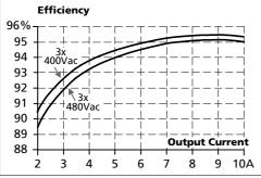
Fig. 11-3 Efficiency vs. input voltage, 48V, 10A
