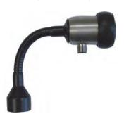
A gooseneck between the electronics head and the primary sensor provides freedom in the orientation of the sensor. This option simultaneously provides thermal decoupling between the two units. The length of the gooseneck is 140 mm.
